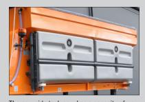
The new side tank now has a capacity of up to 3500 I (small 2200 I, medium 2592 I, large 3500 I) and has been adapted to suit the machine's contours.
