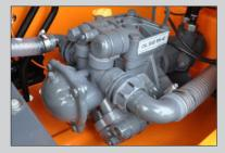
The diaphragm pump for pre-wetting is positioned in the engine compartment where it is easily accessible for inspection. The pump's operation is extremely precise, even after many years of operation.
