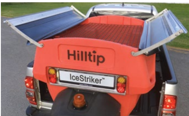
Two-piece tarp mechanism and top screen
