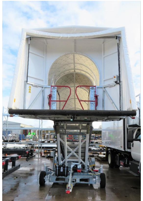
Tristair MR fully covered with interlocked platform safety gates according to EN standard & AHM 913 Controlled Approach System (CAS)
