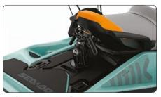
LinQ Retractable Ski Pylon A quick-install retractable ski pylon that stows away when not in use. Features spotter hand grips and rope storage.
